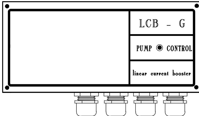
The "LCB - G" pump controller is a high quality DC power converter designed as an interface between a DC (Solar)-Pump (e.g. SHURflo 9300) and a DC power source, like solar panels, wind generators, batteries etc.. The main function of this controller is to maximize the daily water output while providing protection for the pump. The controller can be used in 12V and 24V systems.
